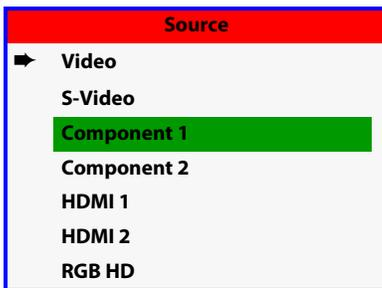
The active source is indicated by an arrow to its left; in this example, Video is the active source. To select a different source, use the ▲ or ▼ button to highlight it and press **ENTER**.
